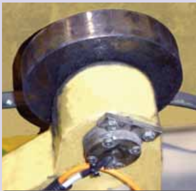
Secondary arm load cell is mounted directly onto the spool reel
